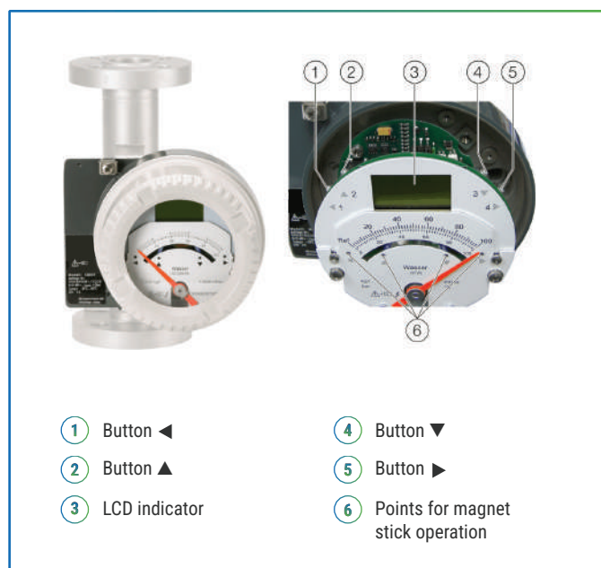
Figure 7: LCD indicator with operating buttons and magnet stick markings
