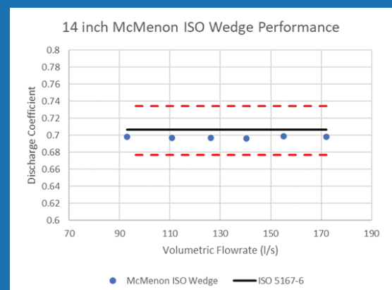
Figure 4: McMenon ISO wedge test results
